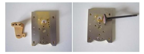
The platform is washed with warm water and the surface rubbed with fine salt using a small wad of clean muslin. A small amount of the Horosilv is placed in a container and using the wet muslin the Horosil is rubbed quickly and evenly over the entre platform. The brass assumes a greyish appearance.
