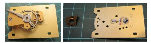
I use a Garryflex medium grit (grey:120 grit) abrasive block to clean the platform and a similar abrasive wheel on a mandrel to clean around difficult areas. The mandrel is held and used by hand. The banking pins are removed and silvered separately.
