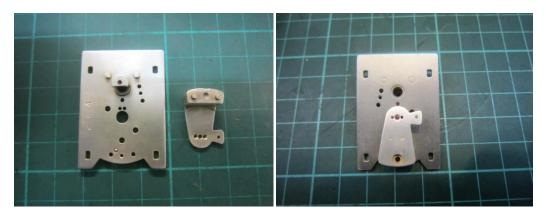
Make sure all holes on the platform are clean before reassembling.
