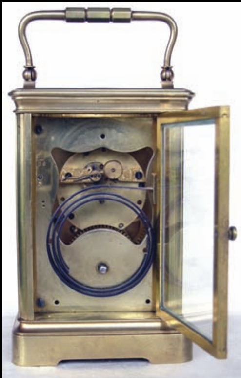
Figure 7. Cyprus model showing damascened backplate, escapement, coiled gong, and hammer.
