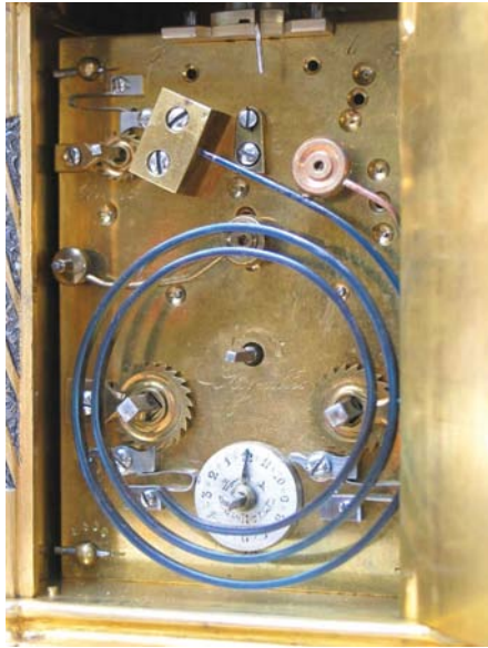
Figure 9, above. The movement back plate showing the internal alarm dial and hand. The tiny alarm disc is engraved in fine detail, with half-hour mark band indications for correct setting. Note the two holes at the top center of the back plate and parallel spring barrel layout. These two traits together are present on many carriage clocks found with the mark of Drocourt.
