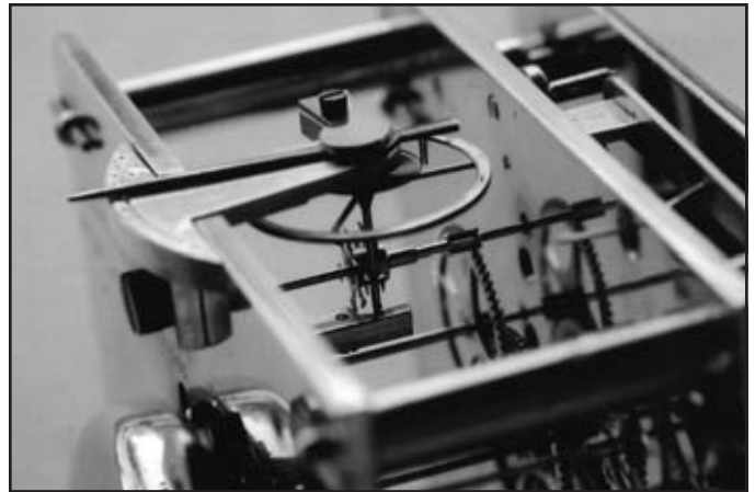
Figure 5. Garnier’s chaffcutter escapement in clock number 1971 shown in Figure 3.
