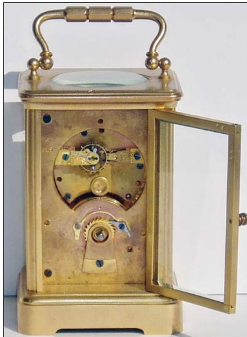
Figure 4. Boston carriage clock, ca. 1887-1888, model Delos (Style 2). Made in Boston, MA. Case: heavy gold-plated brass, beveled glass door and three sides, oval beveled glass on top, gilded mask with porcelain dial, handle similar to many French carriage clocks (this case was made in France). This clock is pictured in the 1890 Boston catalog. Movement: 8-day time only, three gold gilded plates, seven jewels with compensated balance wheel. Size: 6-1/2"h x 3-1/4"w x 3-1/4"d.
