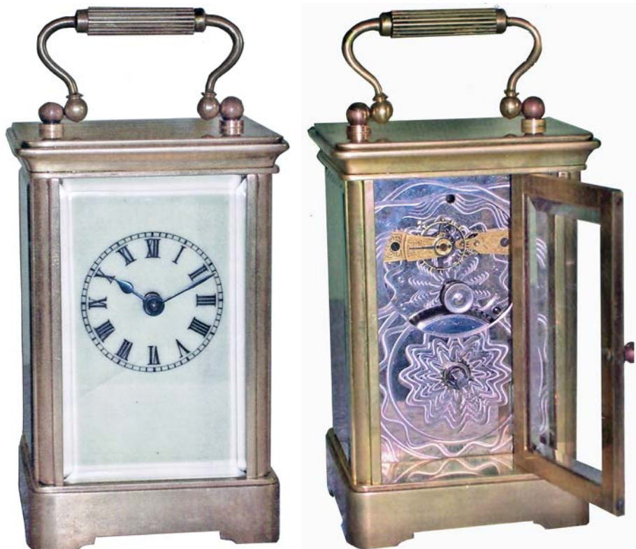
Figure 10. Fair Haven carriage clock, ca. 1897. Made by Fair Haven Mfg. Co. Made in Fair Haven, VT. Case: heavy gold-plated brass, beveled glass door and three sides, full porcelain dial, flat top, multiribbed handle, case similar to Boston "Delos (Style 1)." Movement: 8-day time only, nicked damascene backplate, seven jewels with compensated balance wheel, backplate has a full circle cutaway (which differs from Boston), winding click mounted on the front plate. Size: 6"h x 3"w x 2-3/4"d.
