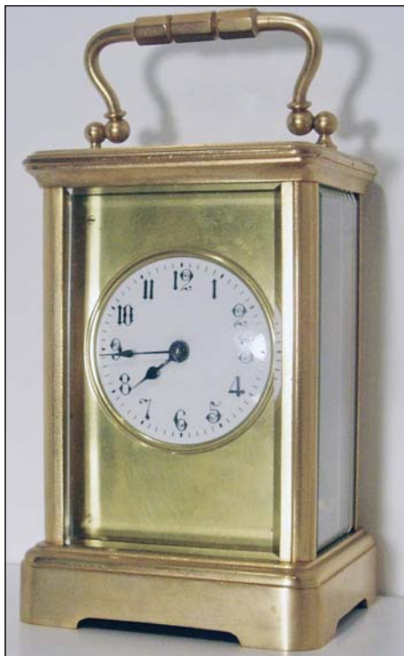
Figure 4. Boston carriage clock, ca. 1887-1888, model Delos (Style 2). Made in Boston, MA. Case: heavy gold-plated brass, beveled glass door and three sides, oval beveled glass on top, gilded mask with porcelain dial, handle similar to many French carriage clocks (this case was made in France). This clock is pictured in the 1890 Boston catalog. Movement: 8-day time only, three gold gilded plates, seven jewels with compensated balance wheel. Size: 6-1/2"h x 3-1/4"w x 3-1/4"d.
