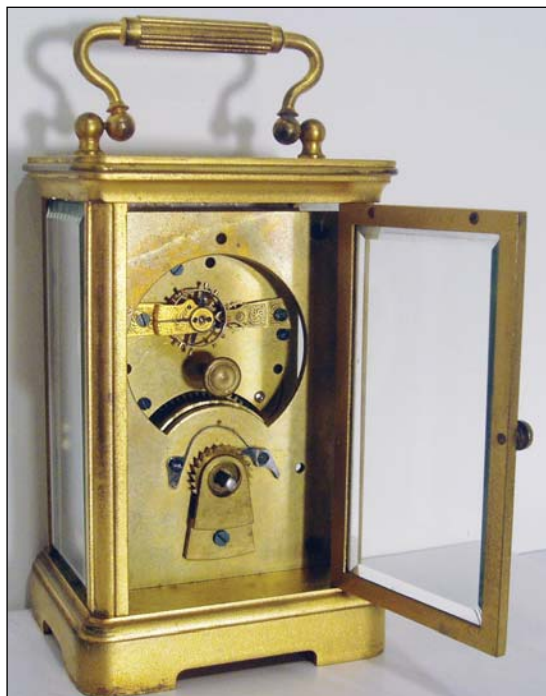
Figure 3. Boston carriage clock, ca. 1884-1885, model Delos (Style 1). Made in Boston, MA. Case: heavy gold-plated brass, beveled glass door and three sides, full porcelain dial, flat top with multiribbed handle, cutaway backplate to view escapement, similar to other Boston carriage clocks (this is the earliest style Boston case). Movement: 8-day time only, three gold gilded plates, seven jewels with compensated balance wheel. Size: 6-1/2"h x 3-1/4"w x 3-1/4"d.
