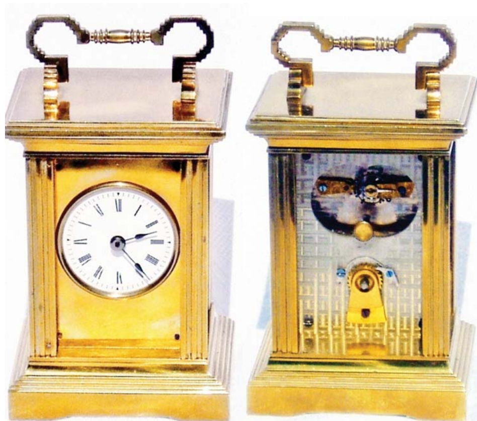
Figure 1. Harvard carriage clock, ca. 1880-1884, S/N 551. Made in Boston, MA. Case: heavy gold-plated brass, beveled glass door and three sides, gold masked porcelain dial, damascene finished backplate. Movement: 8-day time only, three gold gilded plates, 11 jewels with compensated balance wheel. Size: 7" h x 3-7/8" w x 3-1/2" d. Listed with the Chelsea Clock Museum and Harvard Registry. Only eight are known to exist.
