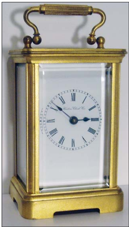
Figure 3. Boston carriage clock, ca. 1884-1885, model Delos (Style 1). Made in Boston, MA. Case: heavy gold-plated brass, beveled glass door and three sides, full porcelain dial, flat top with multiribbed handle, cutaway backplate to view escapement, similar to other Boston carriage clocks (this is the earliest style Boston case). Movement: 8-day time only, three gold gilded plates, seven jewels with compensated balance wheel. Size: 6-1/2"h x 3-1/4"w x 3-1/4"d.
