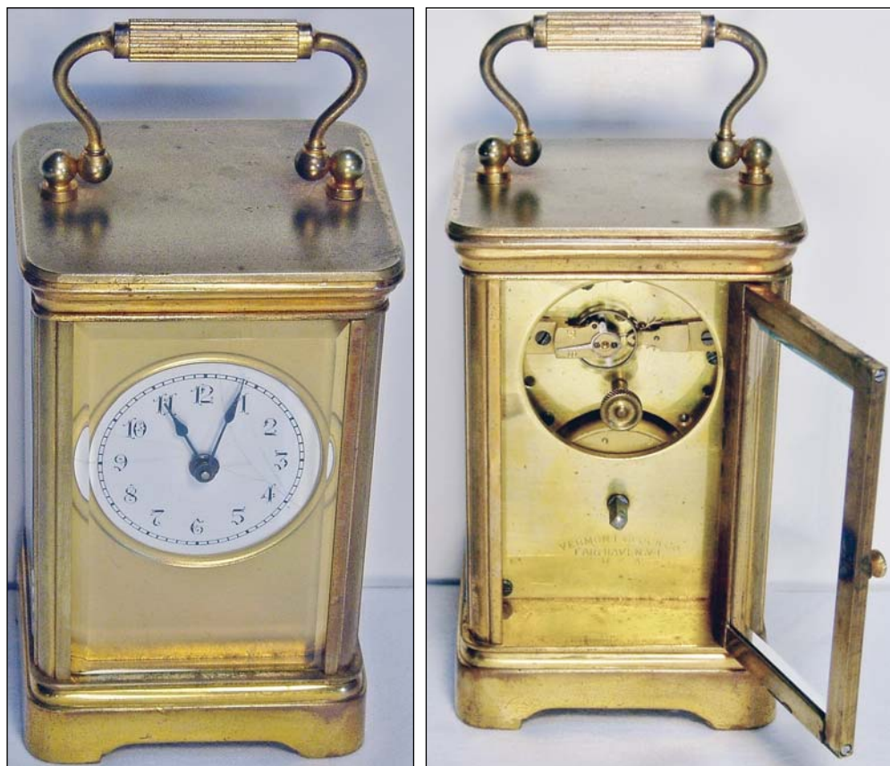
Figure 10. Fair Haven carriage clock, ca. 1897. Made by Fair Haven Mfg. Co. Made in Fair Haven, VT. Case: heavy gold-plated brass, beveled glass door and three sides, full porcelain dial, flat top, multiribbed handle, case similar to Boston "Delos (Style 1)." Movement: 8-day time only, nicked damascene backplate, seven jewels with compensated balance wheel, backplate has a full circle cutaway (which differs from Boston), winding click mounted on the front plate. Size: 6"h x 3"w x 2-3/4"d.
