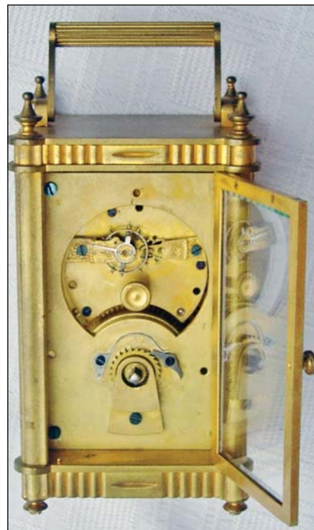
Figure 5, above. Boston carriage clock, ca. 1887-1890, Sparta model. Made in Boston, MA. Case: heavy gold-plated brass, beveled glass door and three sides, gilded mask with porcelain dial, four fancy finials on top, multiribbed handle, bun feet, 3/4 rounded corner posts. Movement: 8-day time only, three gold gilded plates, seven jewels with compensated balance wheel. Size: 6-1/2"h x 3-1/4"w x 3-1/4"d.
