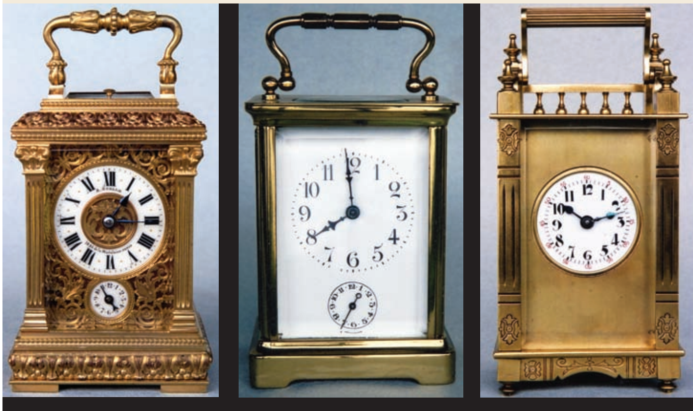
Figure 3, left. French, A. Ecale, numbered 9288, 1-5/8" dial diameter (1-7/8" dial plate width), strikes and repeats, circa 1890. Figure 4, center. French, unnamed maker, not numbered, 1-7/8" dial diameter (2-1/4" dial plate width), timepiece, circa 1890. Figure 5, right. American, Boston Clock Company Queen Anne model, numbered C3767, 1-5/8" dial diameter (2-1/4" dial plate width), timepiece, circa 1890.
