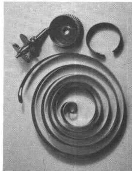
Figure 4. Alarm spring with alarm spring barrel—arbor and slip spring.
