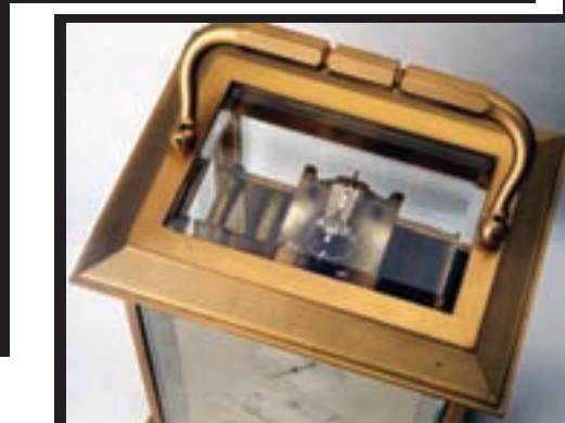
Figure 18. Berthoud, bell strike with seconds hand and 30-minute remontoire, numbered 24. Circa 1860-1870, French, 12" high.
