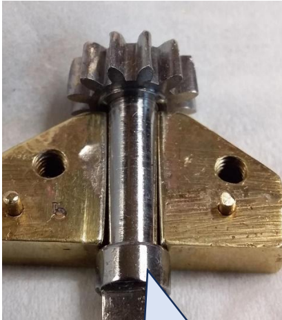
Worn away from vertical, resulting in gear wear.
