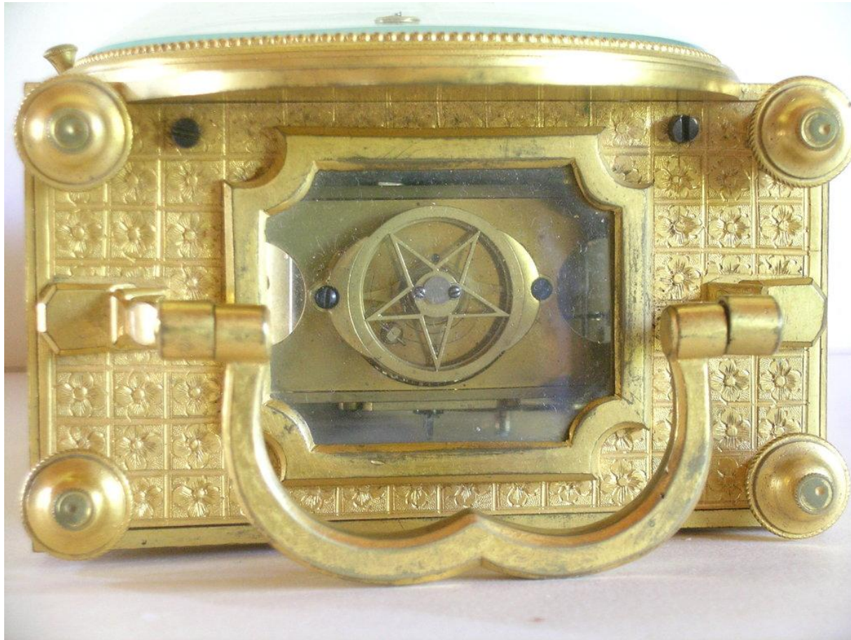
Figure 5. The balance wheel platform and escapement as seen from the top of the clock.
