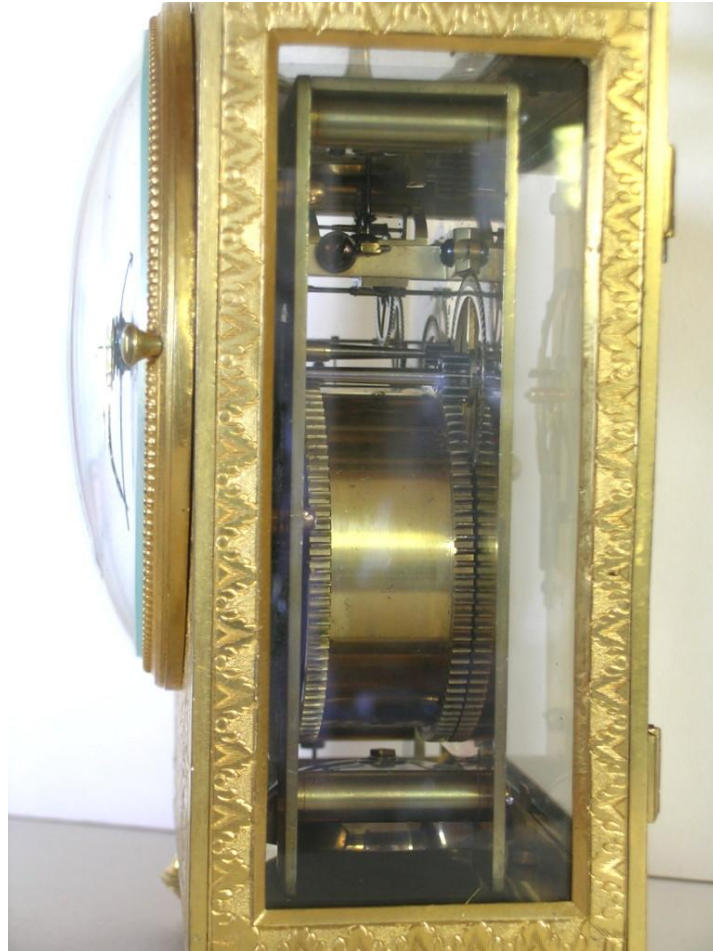
Figure 6. Side view of Duval clock showing the large single barrel.
