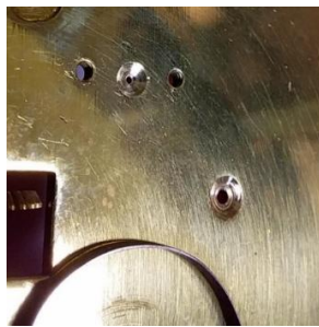
Rebushed pivot holes
