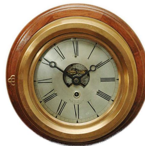
Harvard marine clock SN 1054 c. 1882 6-3/4” diameter Silvered dial w/view window Photo courtesy Jim Dyson
