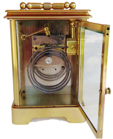
Large Vermont – back view 8-day movement, time & strike on a gong, 2 winding squares, 3 nickeled plates, compensated escapement marked "Vermont Clock Co." 7-1/8"h x 4-3/8" w x 3-1/2" d
