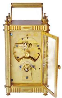
Boston “Sparta” Back view. American case w/ typical ribbed handle. 7 jewel 8-day movement.
