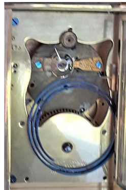
"Cyprus" back view Sculpted back plate. All plates are gold gilded. 8-day movement, time & strike on a gong which is mounted on the back plate. 7 jewels, compensated escapement, single winding square
