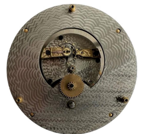
Harvard 8-day movement from marine clock Damascene nicked plates Movement is the same as in the shelf clocks. Photo courtesv Jim Dvson
