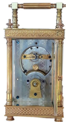
Boston (Fancy Case) Back View SN 1337 Nickered damascene plates, 11 jewel movement, compensated escapement, vertically mounted. Bun feet, glass on 4 sides and top. 6-5/8"h x 3-5/16" w x 3" d
