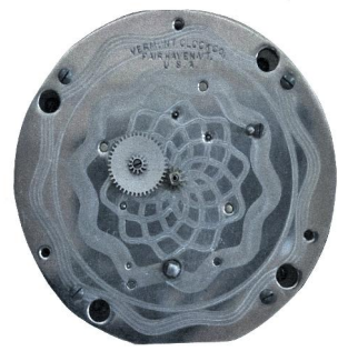
Vermont 5" Marine Clock Movement Damascus back plate 3 nickeled plates, Photo courtesy Jim Dyson
