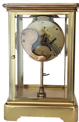
Boston "Crystal" back view Gong holder mounted on pedestal. Tandem wind movement mounted from the top and wound from the front. 8-day, 7 jewel. 9-1/4"h x 6-1/2" w x 5" d
