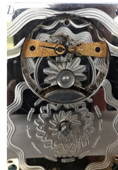
Fair Haven Style 2 Back All plates are nickeled. Movement is the same as style 1 except the damascene pattern is different.
