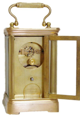
Chelsea (new Boston) Remarked back view. Shows original name circular milled off. 8-day, 7 jewel movement same as most movements from original Boston Clock Co. 6”h x 3” w x 2-5/8” d.
