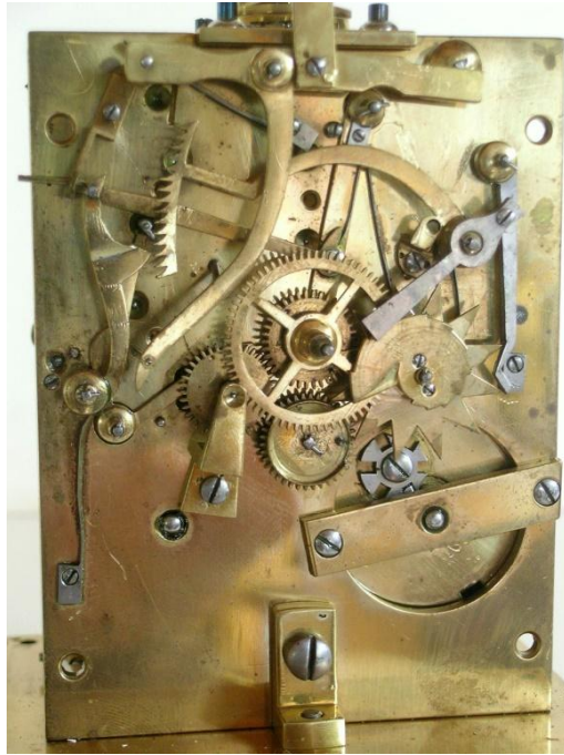
Figure 6. Frontplate of the two-button 5-minute repeater shown in Figure 3a.
