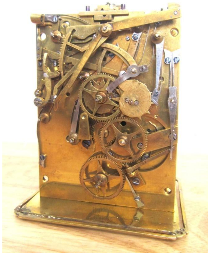
Figure 11. Frontplate of the three-button five-minute repeater shown in Figure 10. (Photo courtesy Stan Boyatzis)
