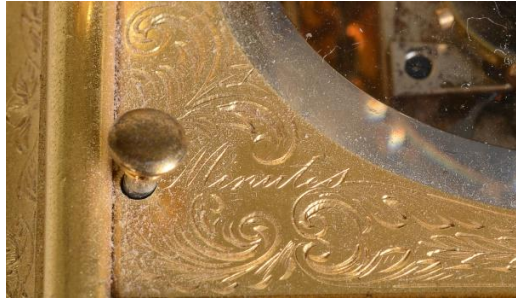
Figure 9a. Front left repeat button with the engraved label "Minutes" (Photo courtesy Dreweatts)
