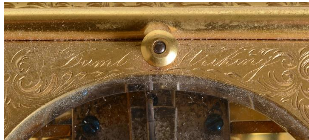
Figure 9c. Back of the top repeat button with the engraved label in two words "Dumb" and "Striking" (Photo courtesy Dreweatts)
