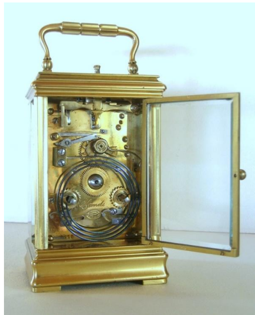
Figure 7. Backplate of the two-button five-minute repeater shown in Figure 3a.
