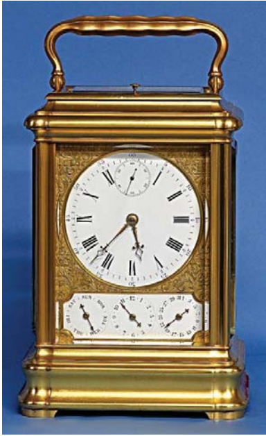
Figure 9. Carriage clock by Drocourt, circa 1895, numbered 12411, with subsidiary dial for seconds at main dial top and subsidiary dials below the main dial for alarm, day, and date (photo courtesy Sundial Farm)
