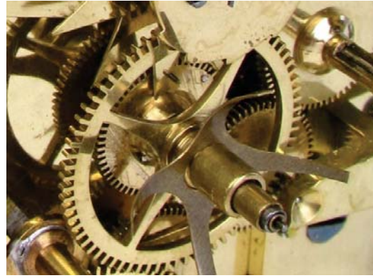
Figure 8. Close-up of the set of arbors on the in Figure 7 that carry the hour, minute, and hands (photo courtesy Leigh Extence).
