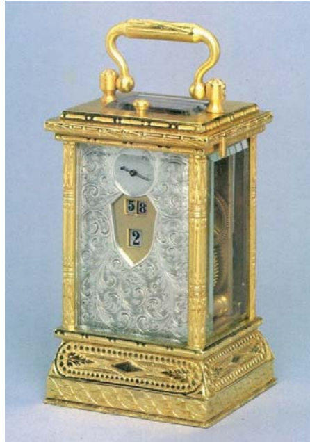
Figure 11. Unnumbered carriage clock by an unnamed Swiss maker with subsidiary seconds dial above the digital main dial (photo courtesy David Nimon)
