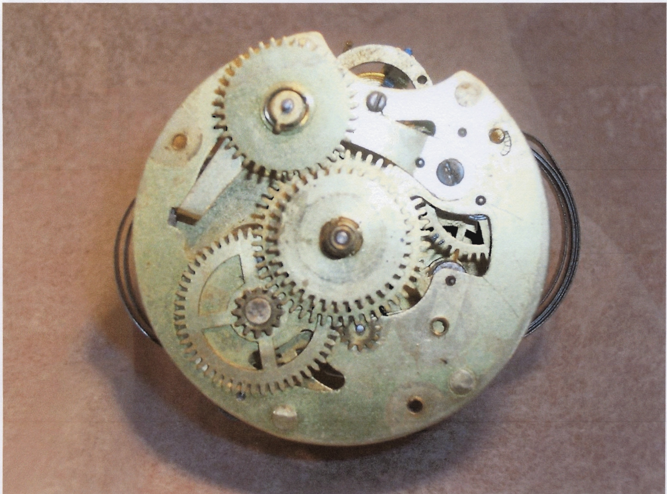
Figure 7 Front view of the movement, The minute shaft does not go through the plate but instead is a hollow tube mounted on a shaft that is riveted to the plate. The hands are set by the small pinion at the 5:30 position and messed with the intermittent wheel.
