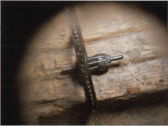
Figure 5 View of the great wheel with solder damage The pinion should be on a clutch so the hands may be set
