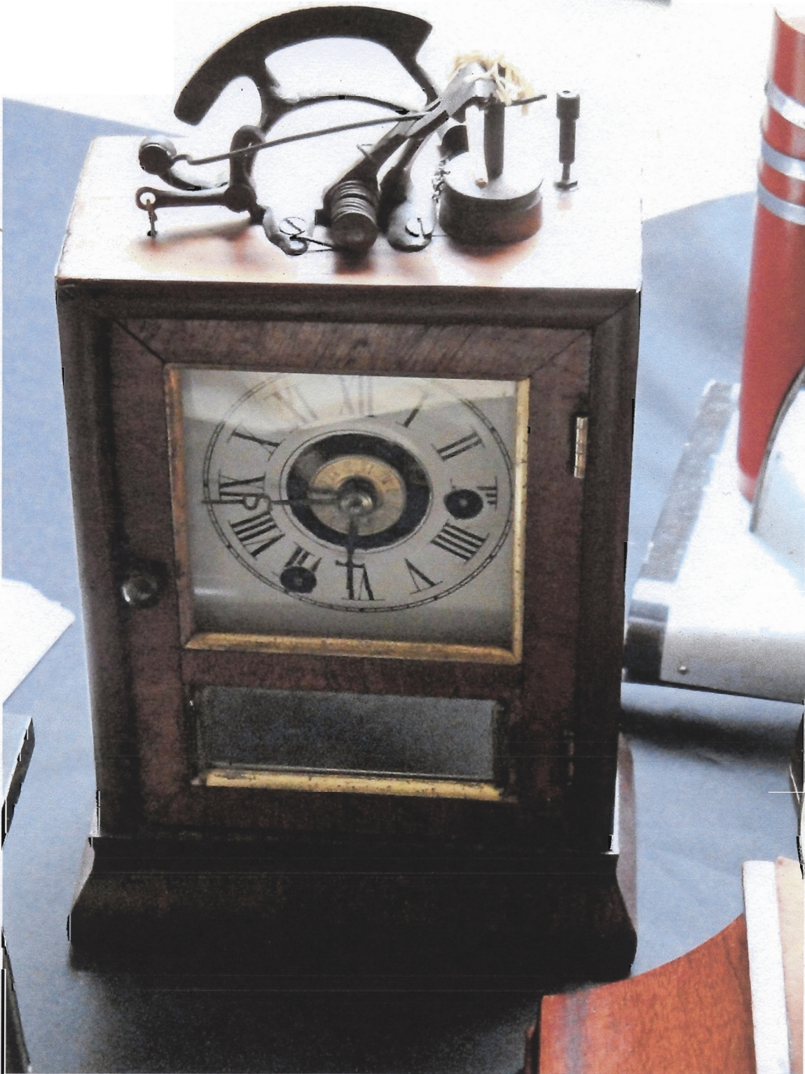
The Seth Thomas Illuminated Alarm Clock ca 1860 (look on the left of the display) The mechanism on the top would strike a match and light a candle when the alarm went off.
