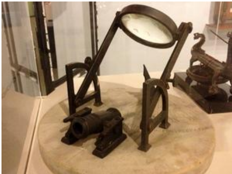
This alarm clock was a sundial that, at the right time, would use a magnifying lens to catch the sun, light a fuse and fire the small canon
