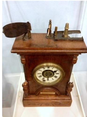
This alarm clock would strike a match at the desired time and light an oil lamp, the idea being that the light would help wake the person up. Unfortunately it would occasionally end up lighting houses on fire.
