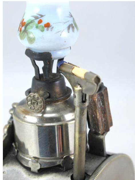
When alarm trips, match strikes flint and then rotates to light mini-lantern wick.
