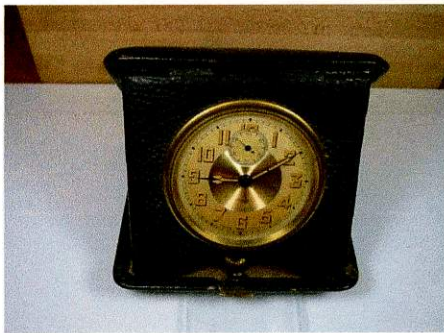
Figure 1 Leaving the realm of Carriage clocks, the need for a light weight well protected clock was met with this leather cased circa 1930 one day alarm inscribed, Norwich Watch Co. Brevet Suisse on the movement. Power for the alarm is taken from the single mainspring.
