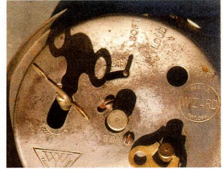
Note slotted holes that allow bell to rotate for loud or soft
