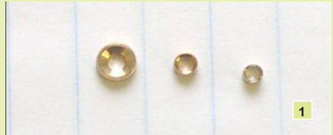
Comparison of commercial and custom made bushings Left Bushing is from Bergeon. Center Bushing is from KWM. Right Bushing is custom made. All have the same hole size.
