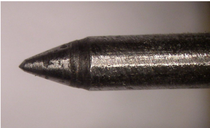
An example of a worn balance pivot, highly magnified. Note the flat spot on the upper tip of the conical pivot.
