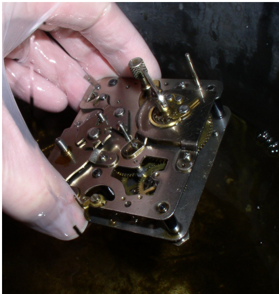
Movement after rinse. Note residue.
