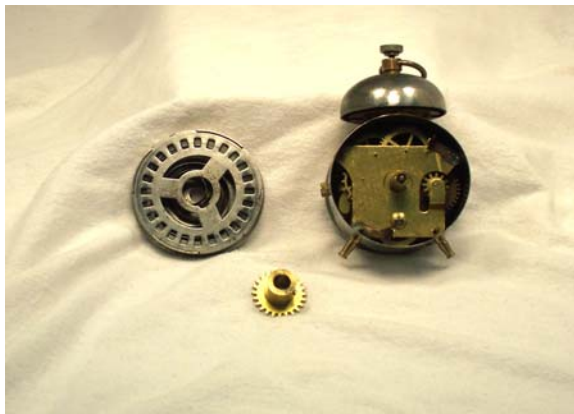
Figure 1: Ansonia Bee Interior At the left is the rear cover of the clock (acting as a mainspring barrel and ratchet wheel). In the center is the main wheel (driven by the mainspring in the barrel shown at the left). At the right, the Ansonia Bee movement with cover and main wheel removed.
