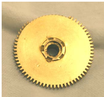
Figure 8: Waterbury main wheel damaged by the sudden uncoiling of a fractured mainspring.
