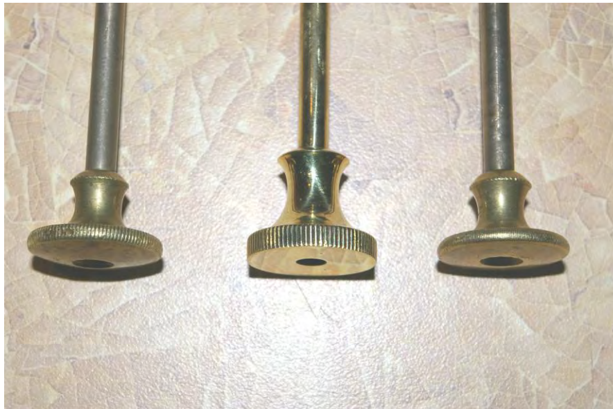
Figure 11. Comparison of the Georg Jacob knurling (center) to other uprighting tool knobs (left & right).
