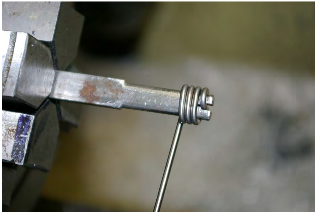
Figure 4. Winding wire on a mandrel to make chain links.
