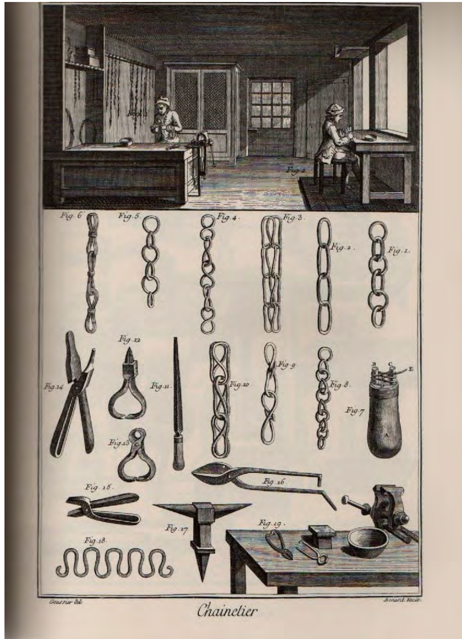
Figure 2. A print showing an 18 th century chain making shop and tools.
