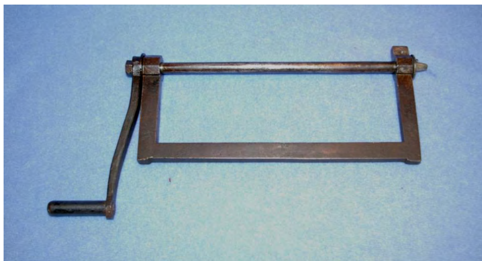
A Clock Chain Making Tool
