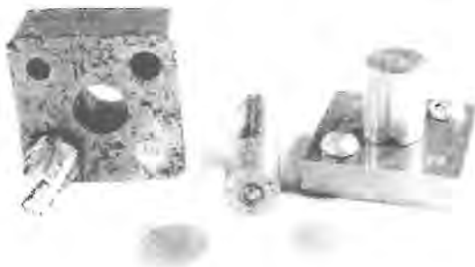
A Saggerson blanking die on the left and a modern example on the right made by the Author to punch-out small escape wheel blank
