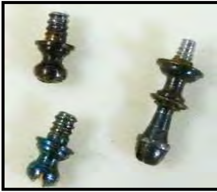
Figure 42: These lovely hand-turned screws with V shaped filed slots were threaded with a screw plate having the characteristic shallow threads.
