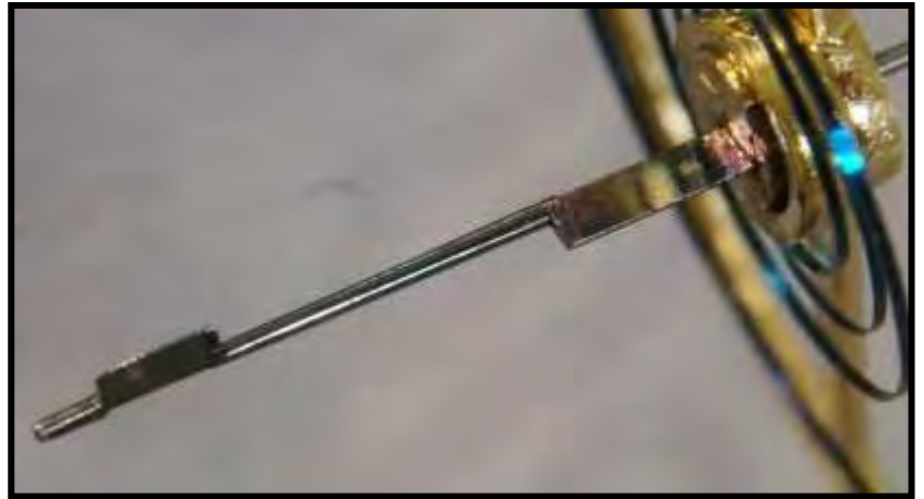
Figure 38. The original staff has practically no wear and is very nicely executed in the classical manner. Notice the rather large upper and lower pivots shown with the very incorrect later period replacement blued and hardened hairspring of approximately four coils.
