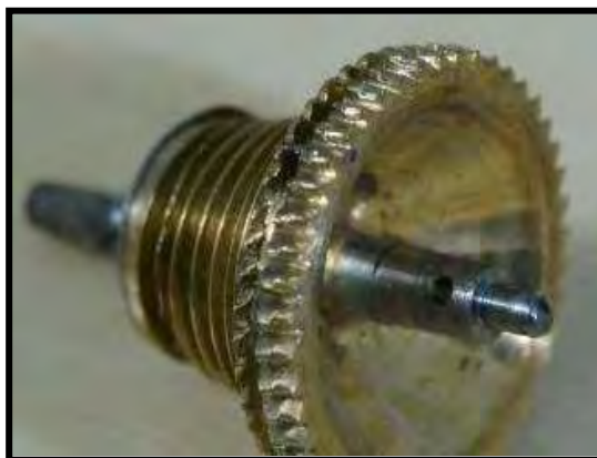
Figure 24 (left): The steel bushing attached to the fusee wheel which if it were extended through the top plate would accommodate a pinion for an hour hand only timepiece.
