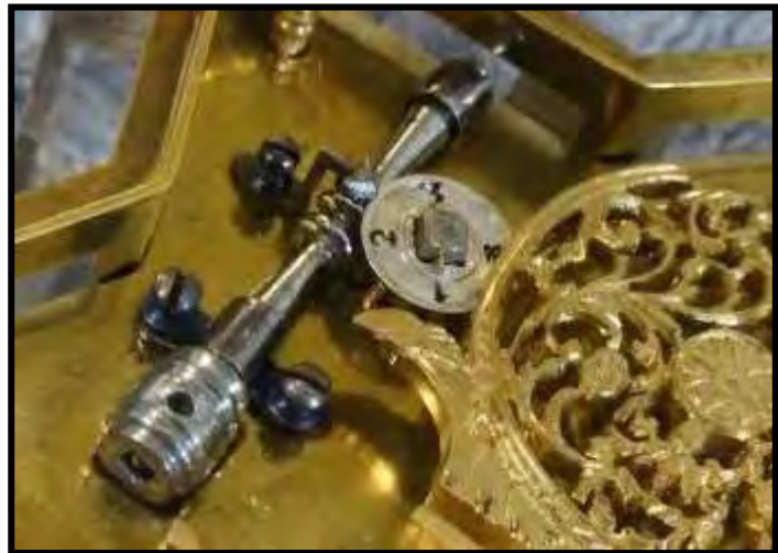
Figure 43 (left): Lower is the Barrow hairspring regulator with the indicator numbers engraved on the back plate, upper is the mainspring setup worm with silver dial. Also seen are the case latches which are found in early English clocks for securing the back plate of the movement the case. Case screws were to be invented many years later.
