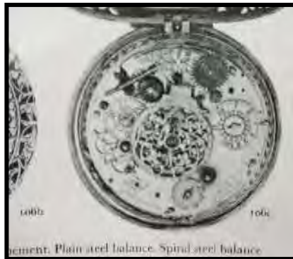
Figure 12 (left): A Daniel Quare of the same period with mainspring setup and Tompion regulators.
