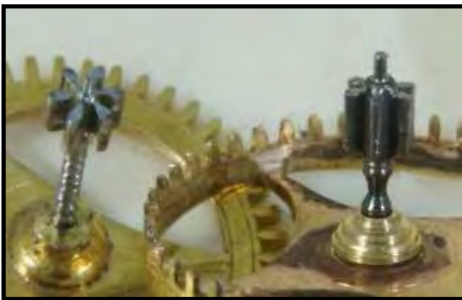
Figure 32 (left): These close-ups of the six leaf “tear drop” pinions beautifully turned arbors and collars illustrate the amazing finish details of this piece. Figure 33 (right): This hand gear cutting is typical of the period with the slightly rounded teeth, pointed addenda and the relieved roots.
