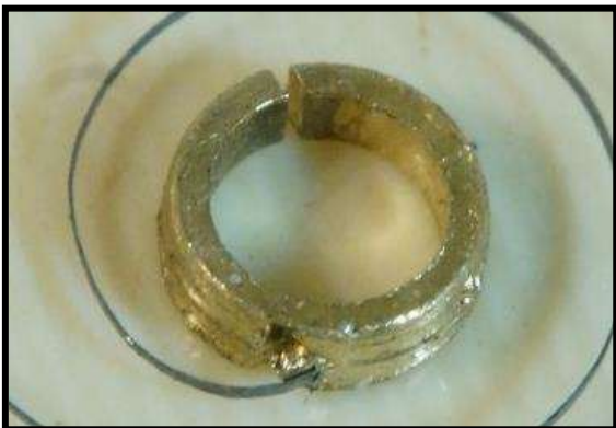
Figure 39: The hairspring in this case is correctly pinned to the outside of the of the collet pin, left to right, if pinned to the inside of the hairspring studding pin the hairspring runs into leading edge of the notch in the collet as well as intersecting the hole for balance hub. The studding pin is also flattened to accommodate the balance hub.
