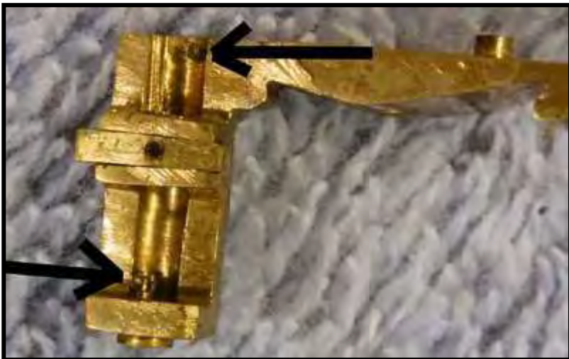
Figure 35: The potence together with the escape wheel centering slide upon close examination (arrows) reveal the two troublesome banking pins. A most elusive and subtle problem that I had never experienced before because it can only occur in a transitional balance timepiece, a period of about ten years. With verge hairspring time pieces overbanking was controlled by a single pin behind the staff opposite the escape wheel.
