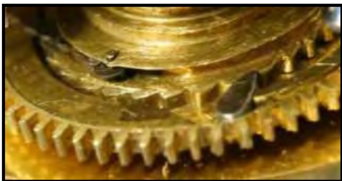
Figure 25 (right): The fusee cord knot hollow persisted even after gut cord was long abandoned in favor of a chain and this style of fusee cannot be used to drive an hour hand as it travels in two directions.
