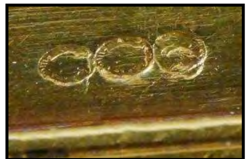
Figures 3 & 4: Assay Stamps. Figure 5 (right): Greatly magnified are the two owls and swan assay stamps in the back of the case, the owls signify gold and the swan stamp for the silver dial. There are no karat designation lines.
