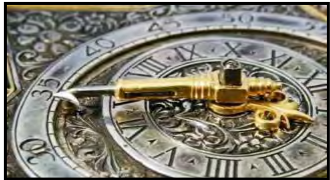
Figure 15 (left): A side view of the tracking minute hand with what appears to be replacement spring, the tracking hand is very sensitive to the spring pressure applied to the tracking roller. Note the hand tracking roller, the replacement extension spring, and the experimental pin hole.
