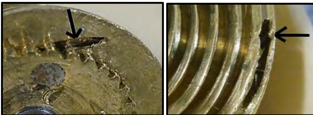
Figure 21 (left): Originally intended for a gut fusee this hole was drilled in the fusee prior to its modification for a fusee to accommodate a chain.
