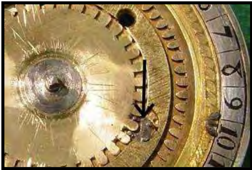
Figure 23: Edward East pre-hairspring calendar watch Ca. 1645 showing the fusee wheel four leaf pinion driving the hour wheel.
