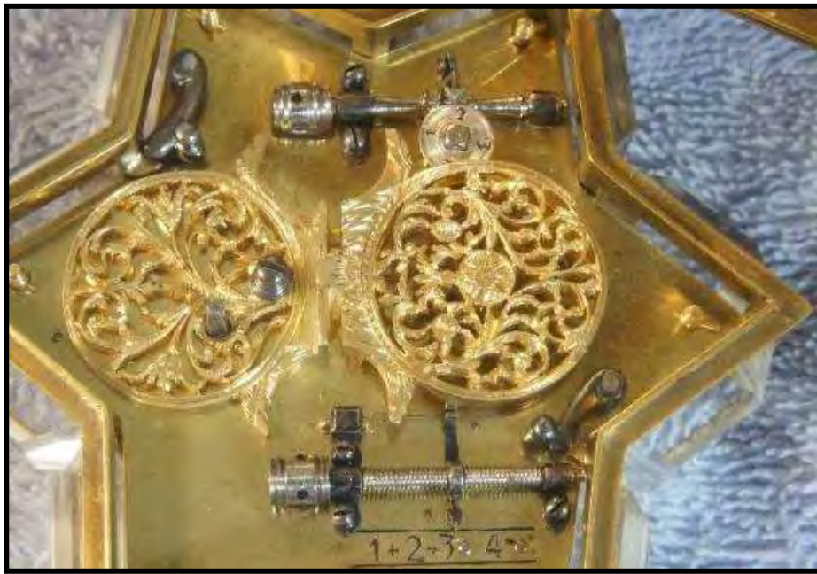
Figure 11: The backside showing the Barrow regulator below and upper mainspring setup worm with a silver indicator dial. Upper left and lower right the nice case latches are seen. The lovely symmetry of the back plate is very much a Breguet style with a balance of mechanical and artistic design and may be the reason the mainspring setup was present even though it was not needed and may account for the choice of the Barrow regulator instead of the Tompion regulator ending up with the lovely artistic visual balanced symmetry.
