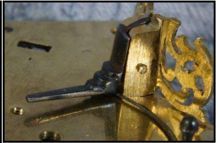
Figure 27 (left): Edward East #3, Ca.1678, with a Barrow regulator is almost certainly his third hairspring watch. The original Barrow regulator was completely missing. The replacement was made by the author. Figure 28 (above): A most elegant fusee iron with a very unusual step design of the Star watch.
