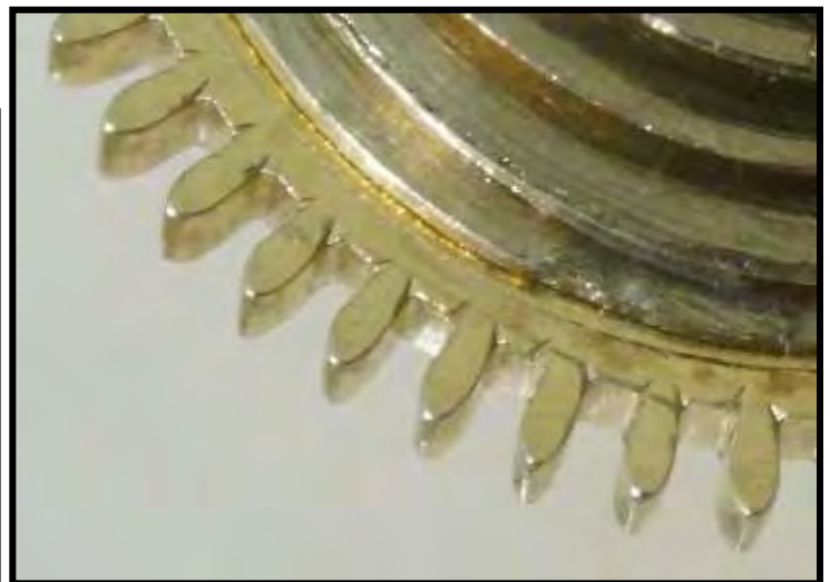
Figure 32 (left): These close-ups of the six leaf “tear drop” pinions beautifully turned arbors and collars illustrate the amazing finish details of this piece. Figure 33 (right): This hand gear cutting is typical of the period with the slightly rounded teeth, pointed addenda and the relieved roots.
