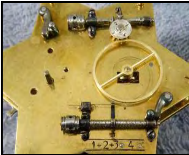
Figure 43 (left): Lower is the Barrow hairspring regulator with the indicator numbers engraved on the back plate, upper is the mainspring setup worm with silver dial. Also seen are the case latches which are found in early English clocks for securing the back plate of the movement the case. Case screws were to be invented many years later.
