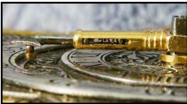
Figure 15 (left): A side view of the tracking minute hand with what appears to be replacement spring, the tracking hand is very sensitive to the spring pressure applied to the tracking roller. Note the hand tracking roller, the replacement extension spring, and the experimental pin hole.
