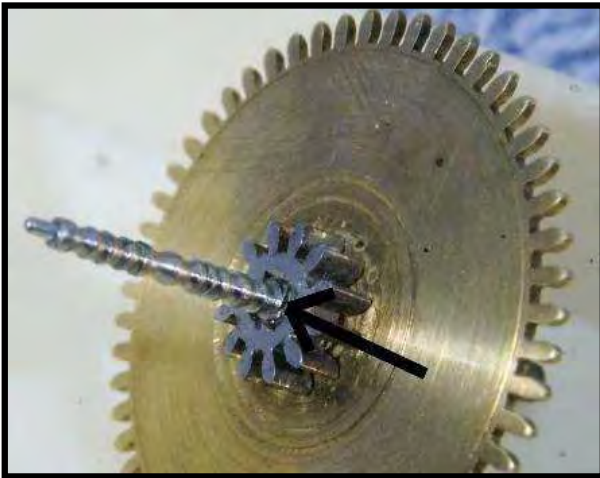
Figure 31: The very unusual square mounting block of the arbor for the center wheel and the separate pinion along with the beautifully turned arbor is an extravagant and unique way of mounting the center wheel.
