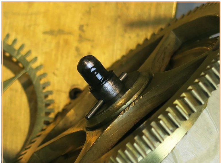
Figure 3 - Barrel and great wheel pivot, blackened lubrication.
