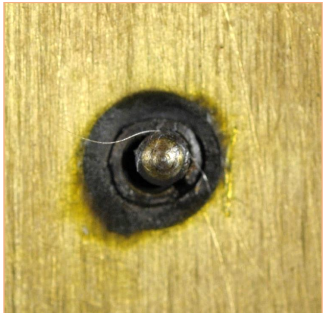
Figure 5 - Dried lubrication on second wheel pivot.
