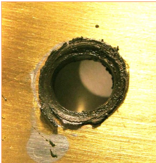
Figure 2 - Dismantling the movement exposes the dried and caked lubrication.
