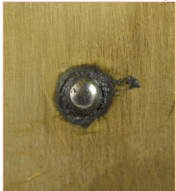
Figure 1 - An obvious problem. Dried and gummed up lubrication on the barrel pivot.
