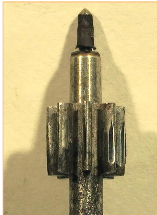
Figure 7 - Second wheel pinion-end pivot. Totally dried and caked lubrication.
