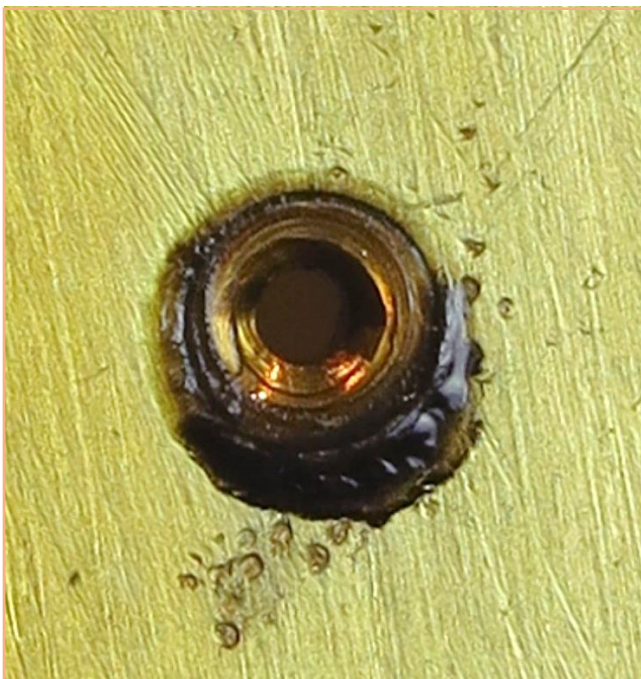
Figure 6 - Second wheel plate pivot hole wheel forced out.
