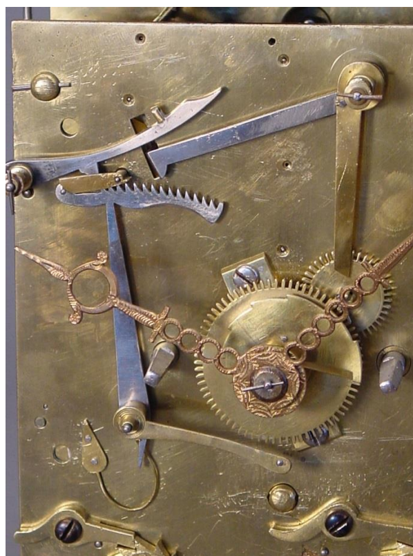
Figure 5 – rack & snail striking mechanism
