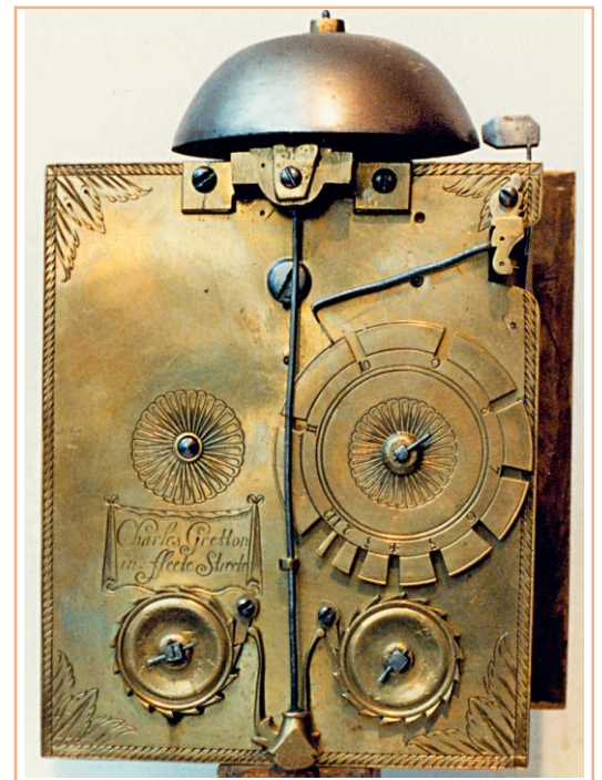
Early short pendulum verge and crown wheel escapement movement with external count wheel strike
