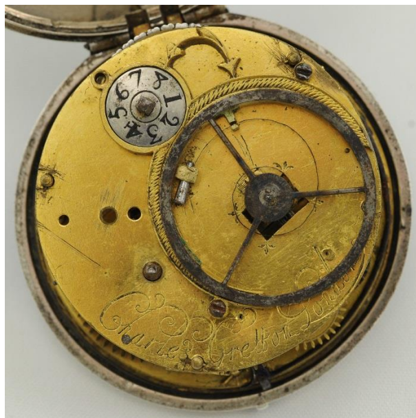
Figure 6 – 17 th century watch with one & half turn balance spring
