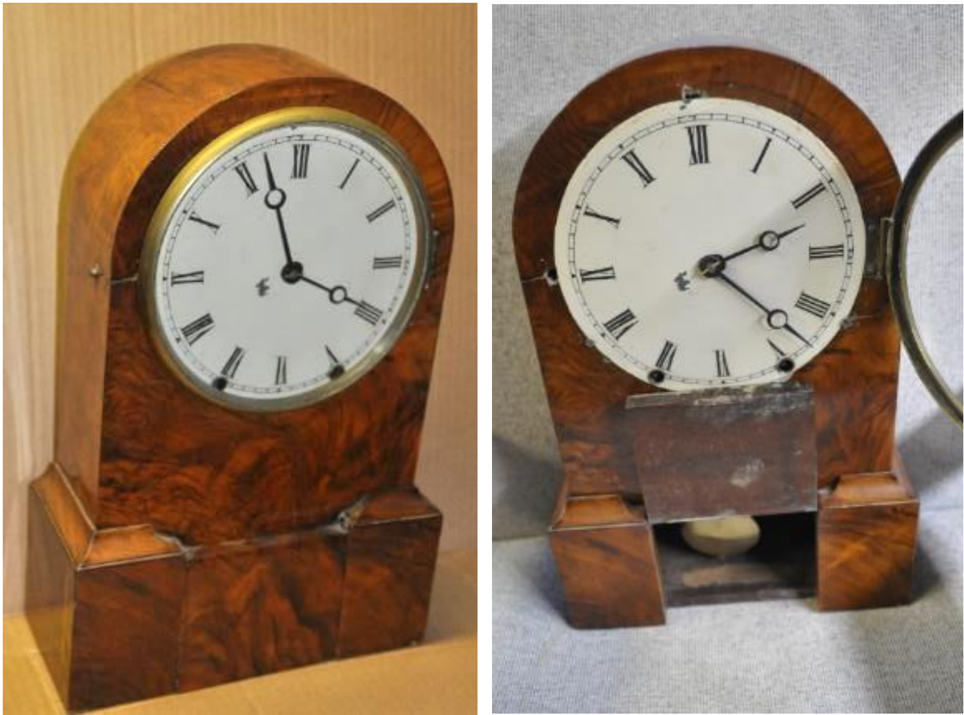
Figure 5: Retailed by Eagle Manufacturing Company, this Anglo-American shelf clock contains a high quality Chauncey Boardman fusee movement. The pendulum is accessed through a clever swing-up door on the front of the case. (courtesy British Horology Chapter member, Safwat Wahba).
