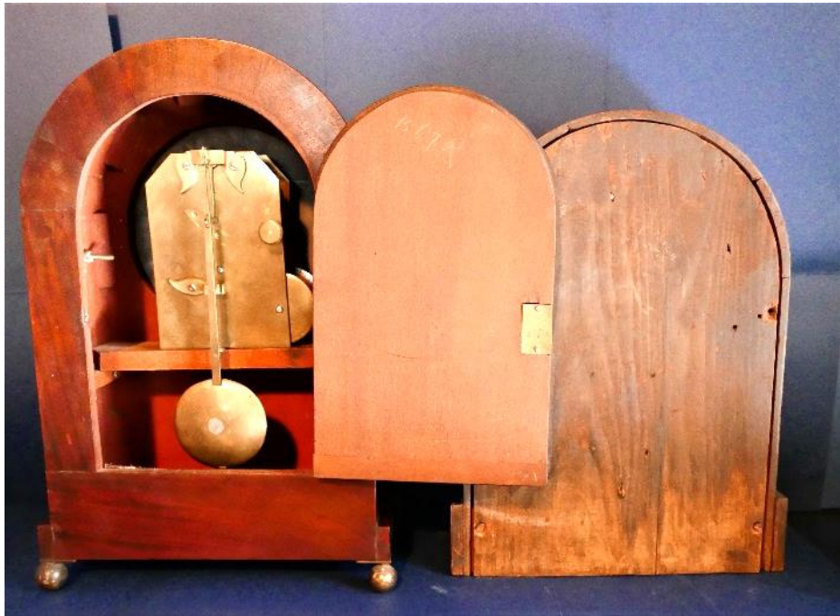
Figure 3: The back of the clocks shown in Figure 2. The English movement bracket clock is on the left (with open door). Its heavy movement is supported by a seat board. The Anglo-American is on the right; no need to spend money on a door. Its light-weight movement is screwed to the backboard and the pendulum is accessed through an aperture cut into the bottom of the case.
