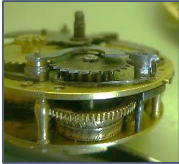
Figure 9: Prototype of the quarter rack and dual pallet for the Lowndes repeater movement
