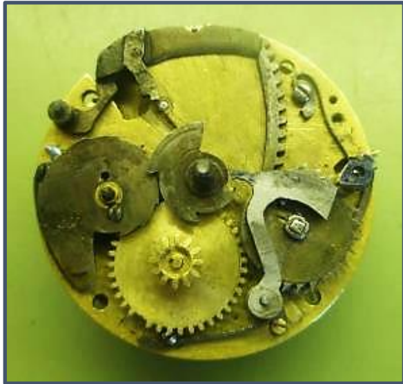
Figure 8: Lowndes Repeater Movement with prototype Quarter Rack
