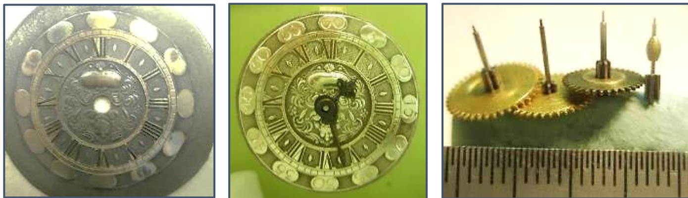
Figure 11: Silver Dial “in The Rough” (left); Figure 12: Engraved Dial with 5 Minute Numbers and Replacement Hands (middle); Figure 13: Replacement runner number 3 – the rate of striking is adjusted by the degree of meshing of the third runner wheel and the mass balanced pinion (right)
