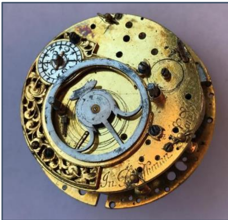
Figure 5: (top) Lowndes Repeater Movement showing peculiar Balance Crossings and Fusee Arbor
