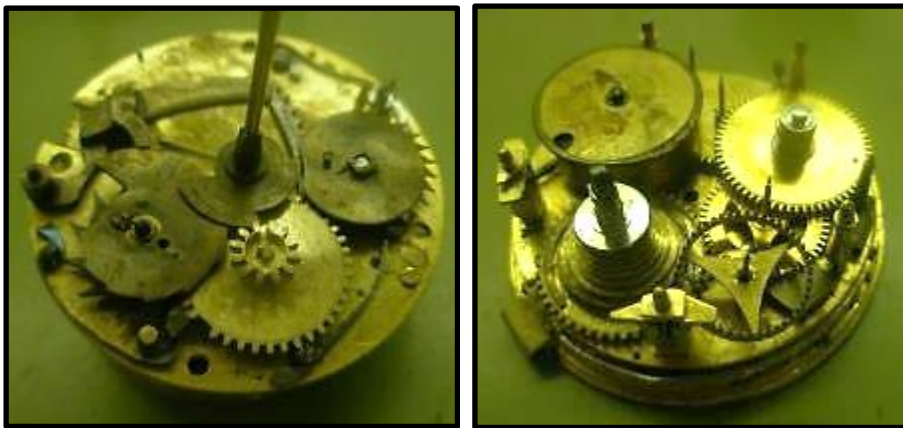
Figure 3: As found under Dial striking mechanism of Lowndes Repeater Movement (left) and missing parts (right)
