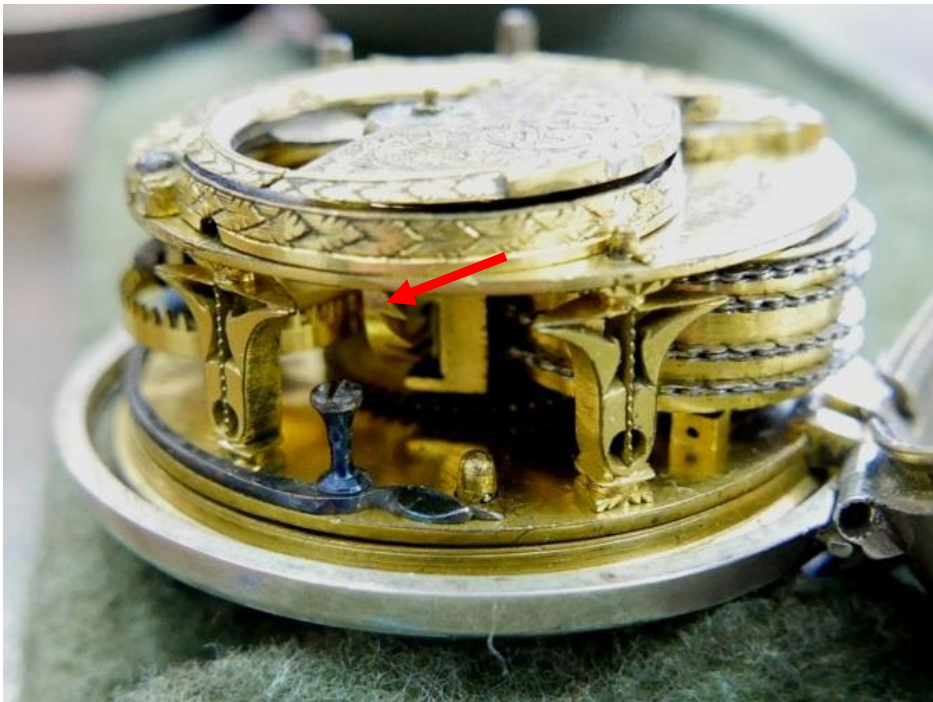
Figure 6: Another picture of the movement showing the intricate tulip designed pillars and the nice engraving around the balance table. Notice the crown wheel that is highlighted by the red arrow.
