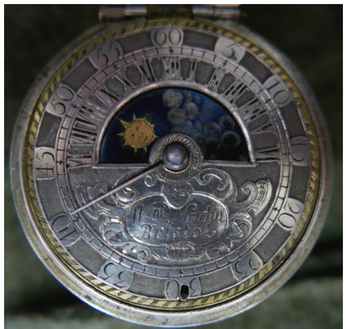
Figure 1: Silver champlévé dial showing moon and stars (left) and sun and clouds (right) animation that turns once in 24 hours. The single hand points to the minutes. The watch is key set, as were all English watches at the time, by turning the squared center arbor with the same key used to wind the watch.
