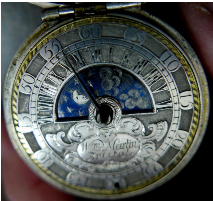
Figure 1: Silver champlévé dial showing moon and stars (left) and sun and clouds (right) animation that turns once in 24 hours. The single hand points to the minutes. The watch is key set, as were all English watches at the time, by turning the squared center arbor with the same key used to wind the watch.
