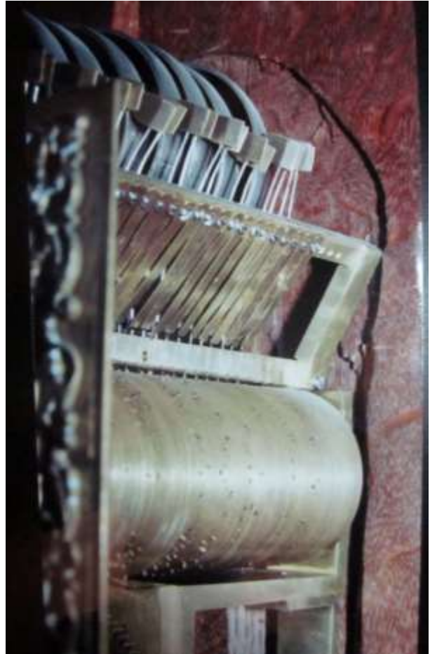
Figure 6: Pin barrel with 20 hammers and 9 bells above
