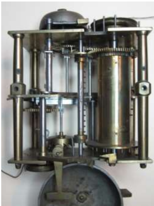
Figure 6: Front of the alarm and pull quarter repeat mechanism with the companion time movement removed. The pull repeat is on the top right with the quarter bell adjacent. The hour is rung on the bottom bell that also doubles as the alarm.
