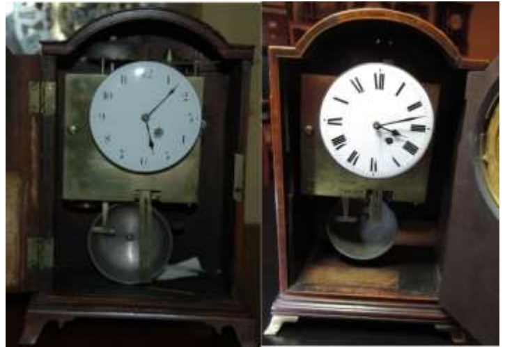
Figure 3: Inside of the clocks in Figure 2 showing nearly identical movements. The movement is signed: "TRUSTED'S PATENT REPEATER / WM. BARTLEET BIRMINGM".
