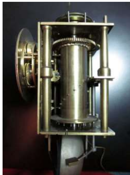
Figure 7: Right side of movement showing the pin barrel that controls the hour strike. A plate (not visible) between the timepiece and the strike mechanism allows easy adaptation of different timepiece movements. This photo has the time movement reattached to the alarm and quarter repeat mechanism frame.
