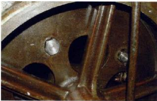
1. Rear view of hour strike barrel. Bolt heads were rubbing.
