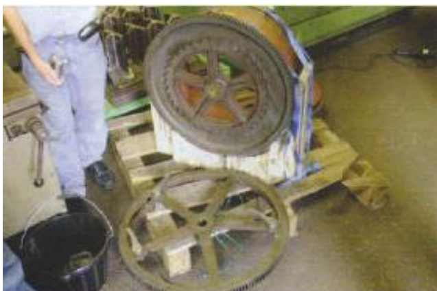
17. Going barrel before bush and washer replacement.
