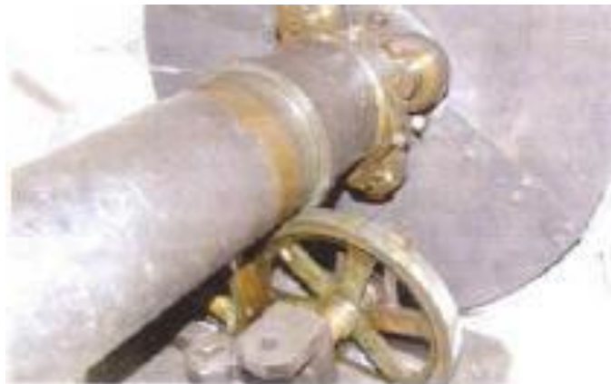
14. Friction rollers behind the dial.
