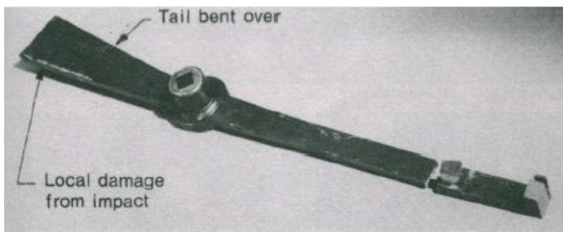
Fig. 4b. Chime locking lever, overall view showing bent counter-balance tail.
