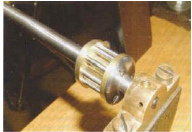
22. Finished lantern pinion with new trundles.
