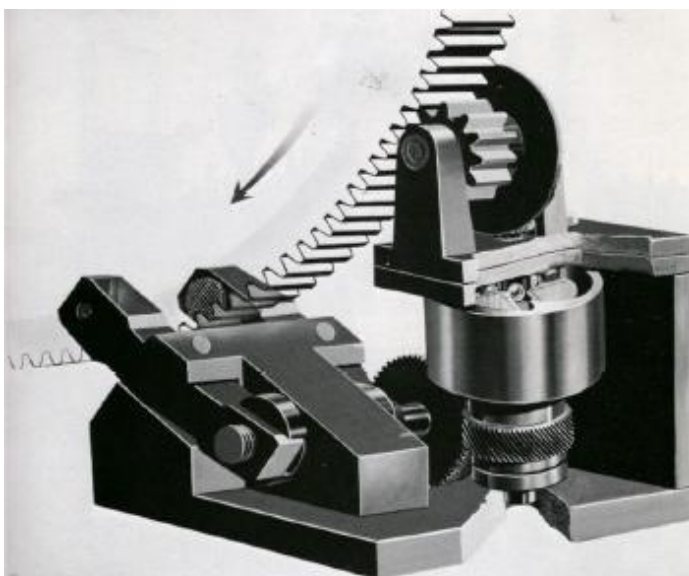
Fig. 12. Inertial safety brake installed on both strike main wheels.
