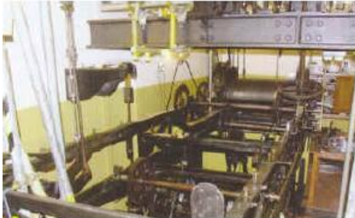
18. Clock frame stripped of parts, ready for inspection.
