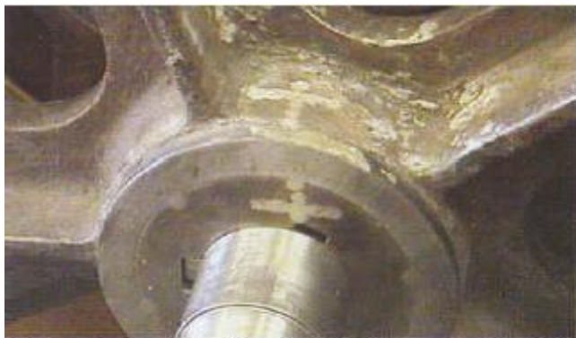
16. Repair using cold stitches that look like a row of filled holes.
