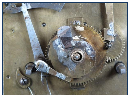
Figure 2: Detail of the rack striking control (above)
