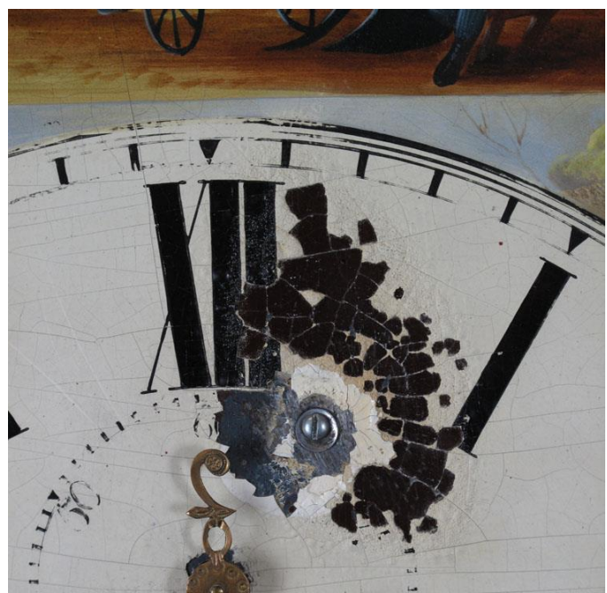
Figure 6: Dial as received with detail of flaking damage (two images)
