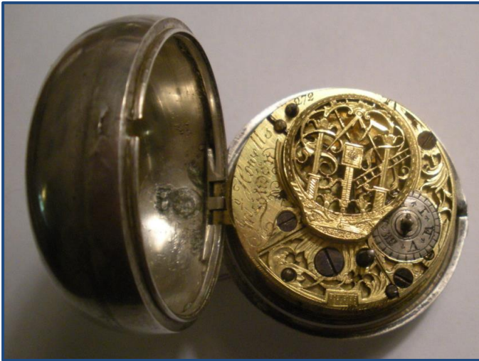
Figures 2-3: Movement of John Howells watch with close-up of the balance table on right
