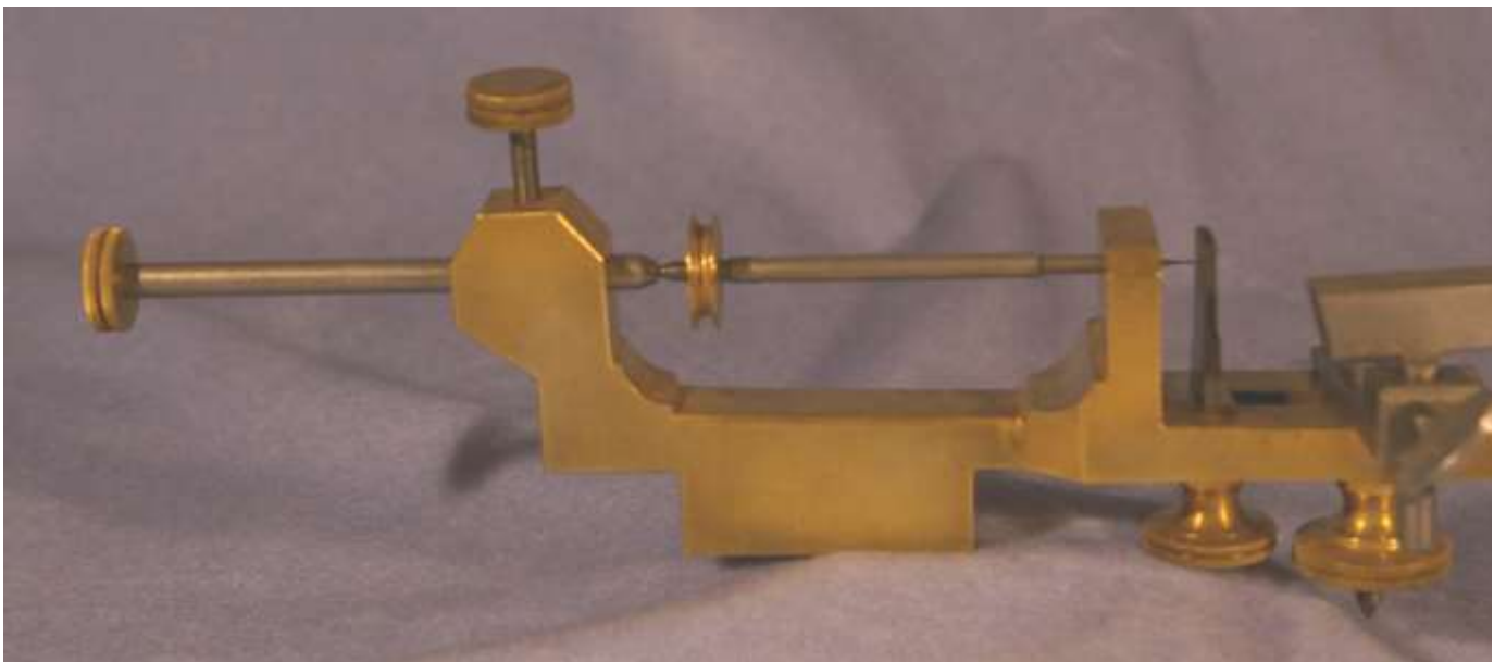
Figure 4. Lathe possibly modified for repivoting
