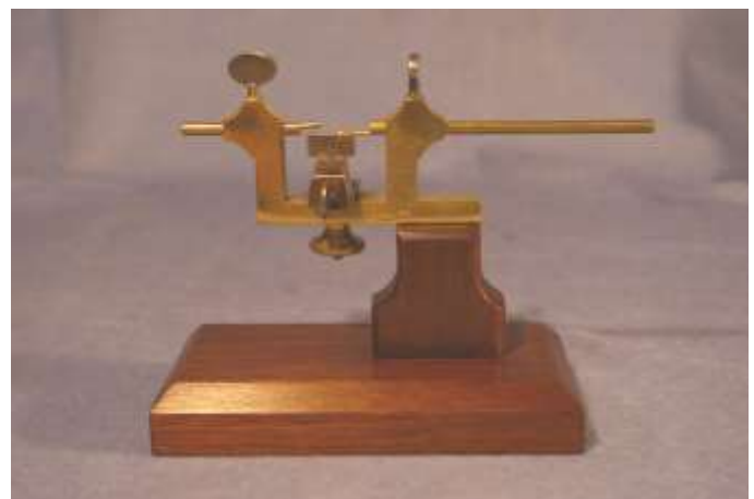
Figure 1. A simple brass turns marked "W.S" on the body
