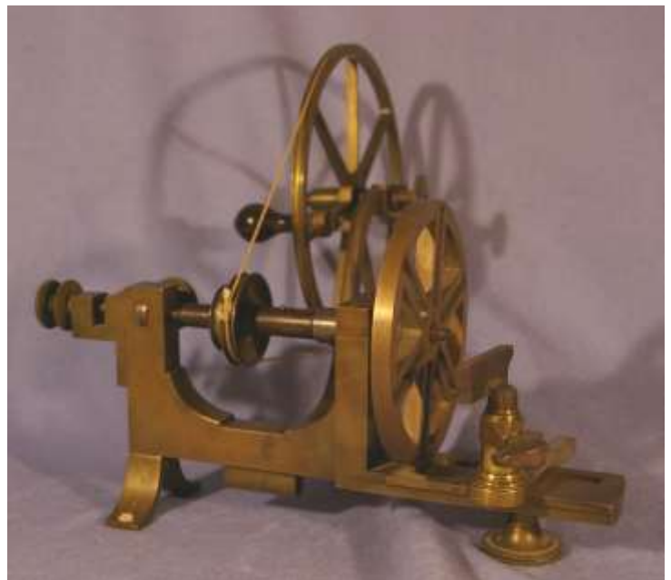
Figure 8. A Henry Leyland mandrel lathe
