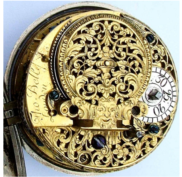
Figure 1: Tho. Bell, London, verge showing intricately engraved and pierced balance table
