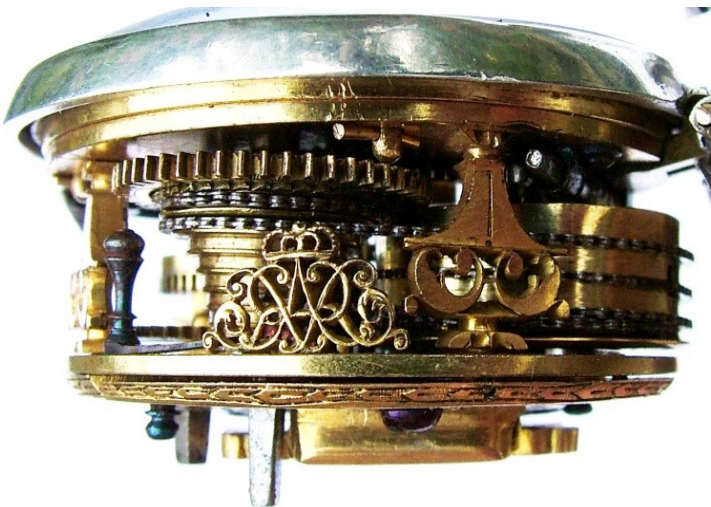
Figure 2: Side view of Bell watch showing Egyptian pillars with pierced gallery and Royal cypher for Queen Anne, circa 1705
