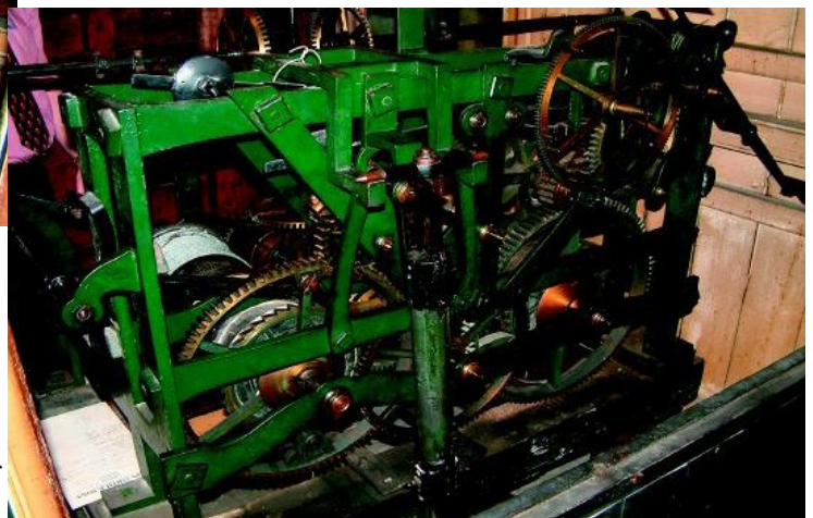
Below: Movement from the rear. The pendulum rod is wood. Bushes are fitted with oil holes.
