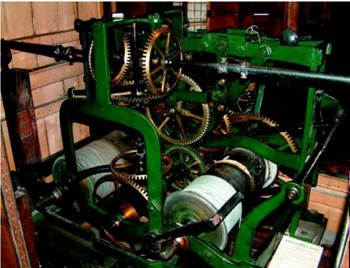
Left: Holmes' movement from the front. The going train is on the right. Maintaining power by bolt & shutter. Note the tied-up striking release lever.
