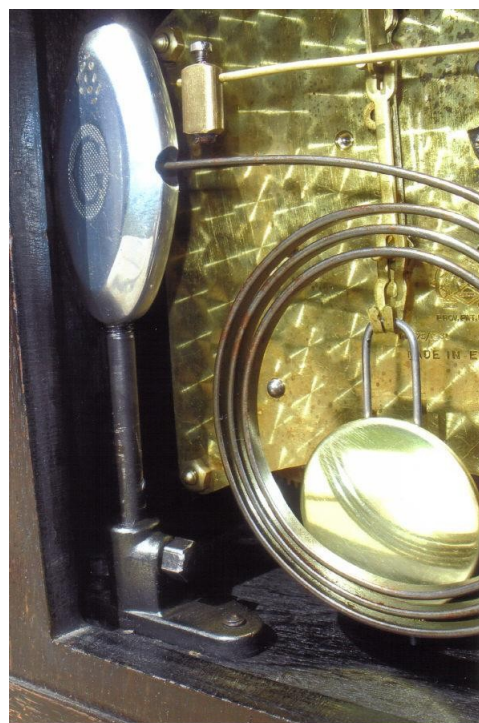
A view of the gong unit with the "G" visible. Note the nice engine turning on the plate.
