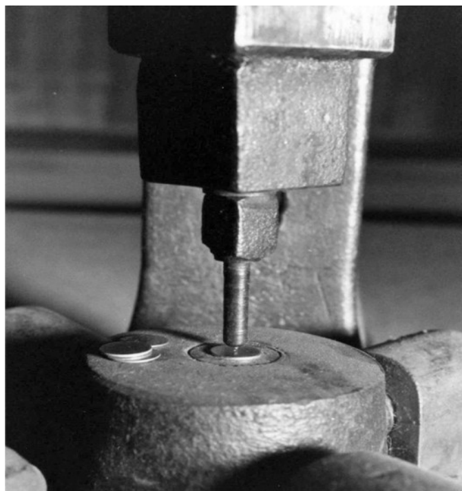
Figure 5. A fly press punch used to make the center hole in the wheel blank.
