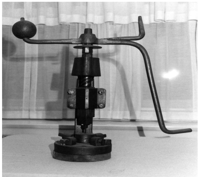
Figure 10. Ball and fly press used to punch center holes in wheel blanks.
