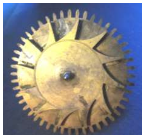
Figures 9-10: Front and back views of the dial wheel showing replaced teeth. Notice the scribe lines on the photo to the right that marked out the 12-pointed star for the strike trip.
