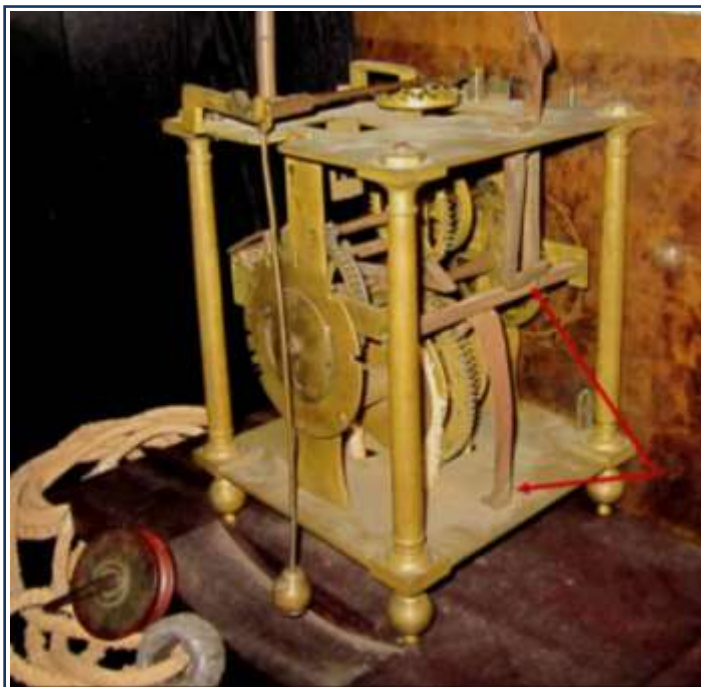
Figure 7: (left) Tall case movement with decorative line designs on the hammer spring and stop highlighted. Notice the outside count wheel on back. Likely original wooden pulley and lead counter weight shown can be seen in the foreground. Figure 8: (right) Close-up of knife-edge verge escapement and escape (crown) wheel.
