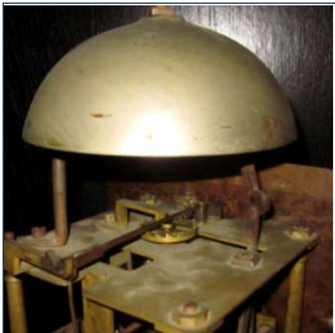
Figure 7: (left) Tall case movement with decorative line designs on the hammer spring and stop highlighted. Notice the outside count wheel on back. Likely original wooden pulley and lead counter weight shown can be seen in the foreground. Figure 8: (right) Close-up of knife-edge verge escapement and escape (crown) wheel.
