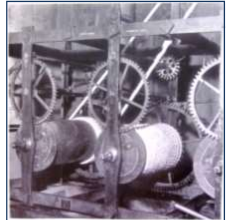
Figure 1: Windsor Castle's three-train turret clock; the time train is in the center. Inscribed "JOHN DAVIS WINDSOR 1689" (courtesy of Country Life).
