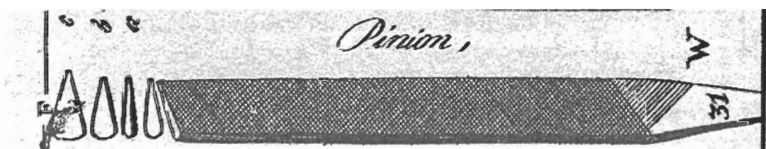
Fig. 4. A pinion file from ca 1790.
