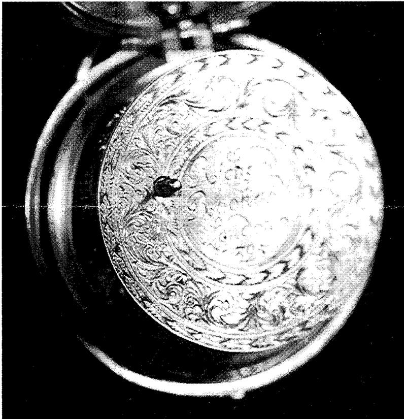
ENGRAVED TOP PLATE WITH PROTRUDING WINDING ARBOR, ROOKER NO. 325
