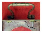
other side of the handle. That is visible in the photo (see the adjacent photo). The free end of the spring also serves as a lever to press down against another lever in the movement to inhibit the alarm from sounding. This appears to be working, but will have to be verified when the movement and clock case are joined after servicing. It may still need some alignment and adjusting.
