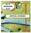
The movement has solid plates on, front and back, so the positions of the pallets relative to the teeth on the escape wheel were not easy to see. Visual observation was not clear enough to accurately determine the operation of the escape wheel and pallet assembly, but I concluded that to properly adjust the drop and lock
