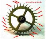
with crooked teeth. To straighten the teeth, I used a pair of flat nosed pliers to pull and straighten each tooth. This results in stretching
