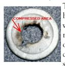
The shaft/pulley end of the motor is held centered by a soft plastic spacing washer. As the motor, and its shaft move closer to the sound disk it binds on the collar. The stalled motor will drain the battery. The binding is shown in the photo with a bamboo
