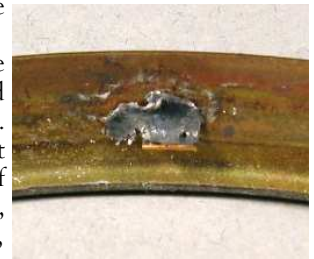
Poor solder job
