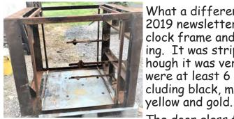
What a difference a few months can make! The January 2019 newsletter featured early photos. See the Lockport clock frame and parts before sandblasting and powder coating. It was stripped to the bare frame, although it was very rusty it is salvageable. There were at least 6 coats of paint on most parts, including black, medium blue, dark blue, cream,
