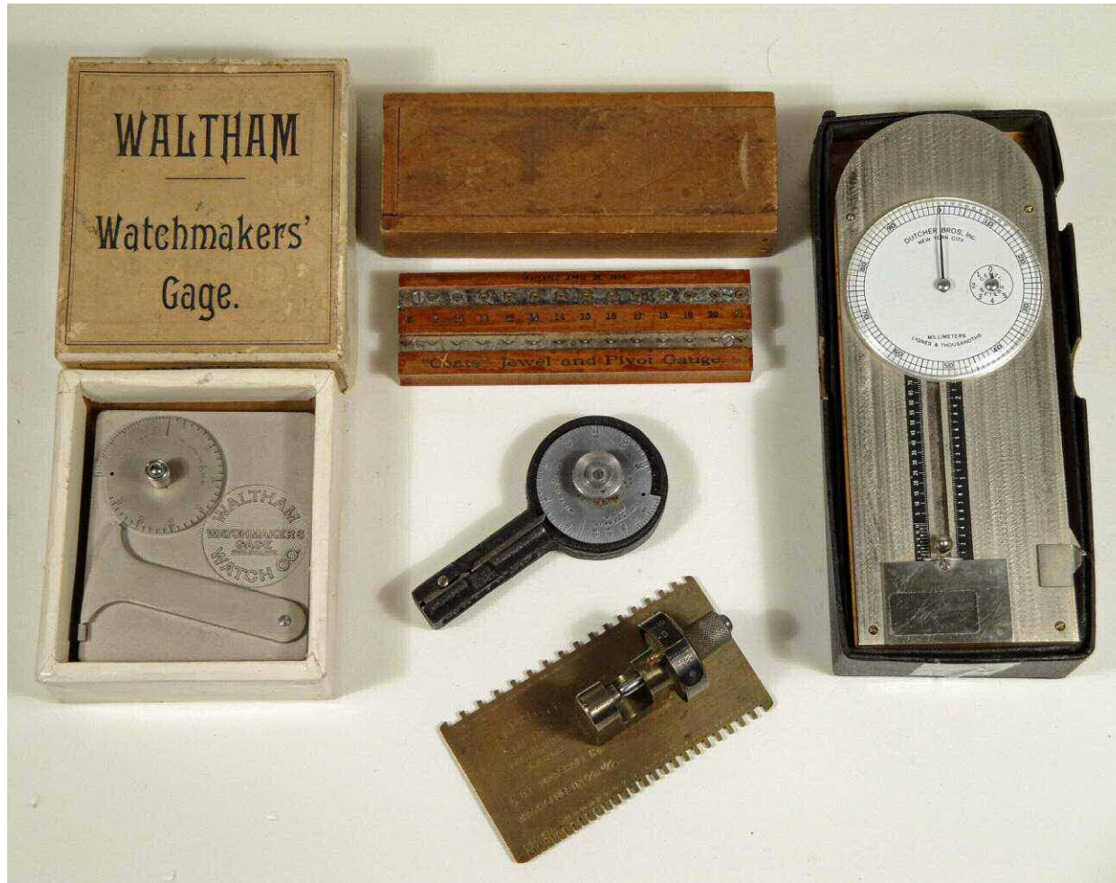
Assortment of gauges for mainsprings, Jewels, Pivots and Watch crystals
