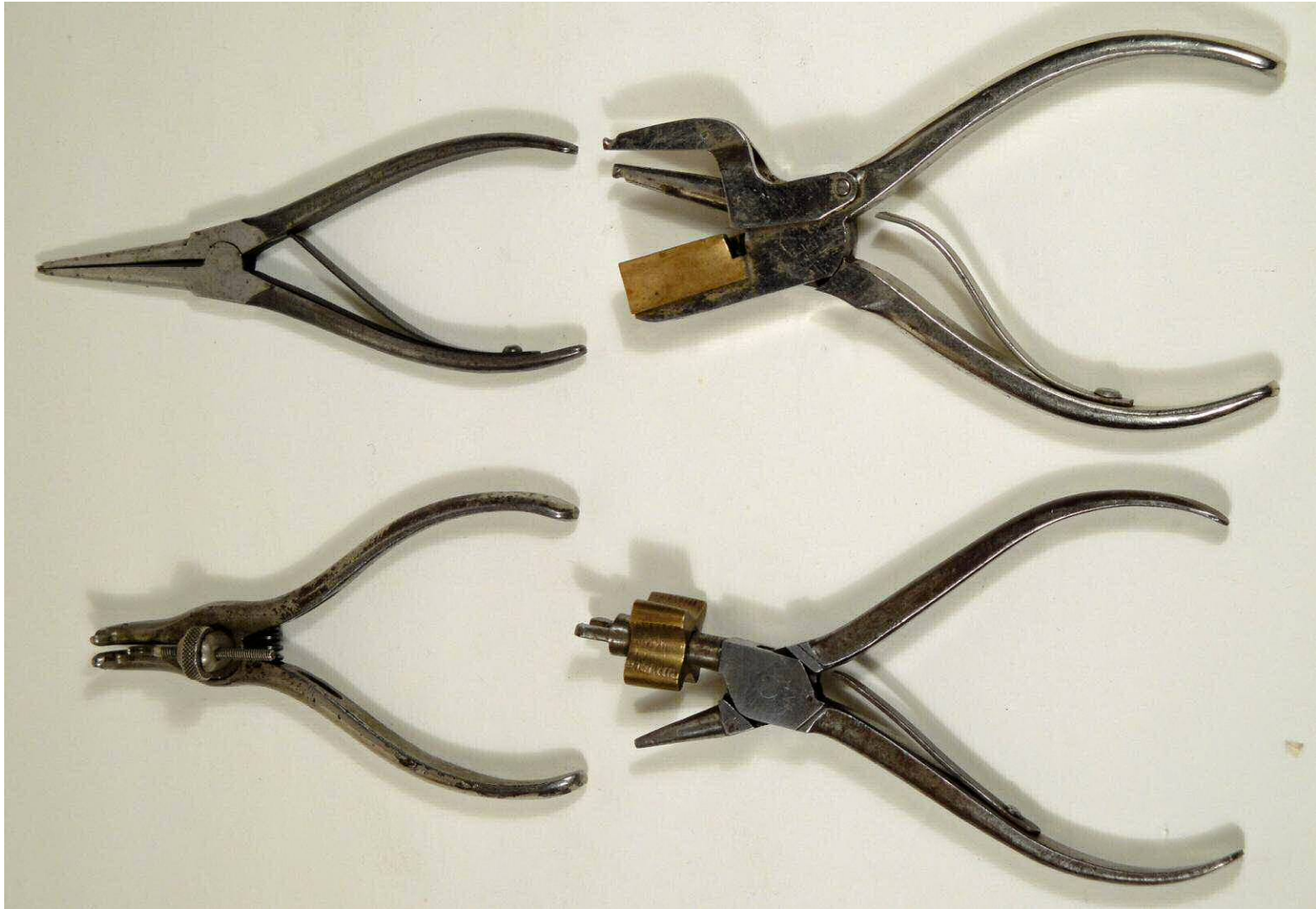
An assortment of watch bow opening and closing pliers
